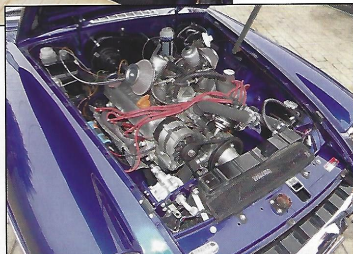
The torque of the V8 is an increase of 80 per cent over the standard four-cylinder, making it easy to drive with performance being available from low engine speeds in any gear.
